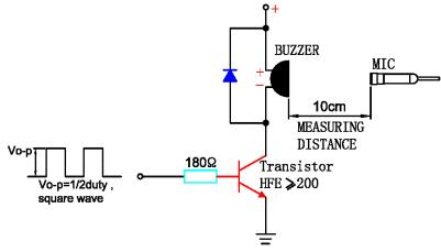
In the measuring test, buzzer is placed as follows:
