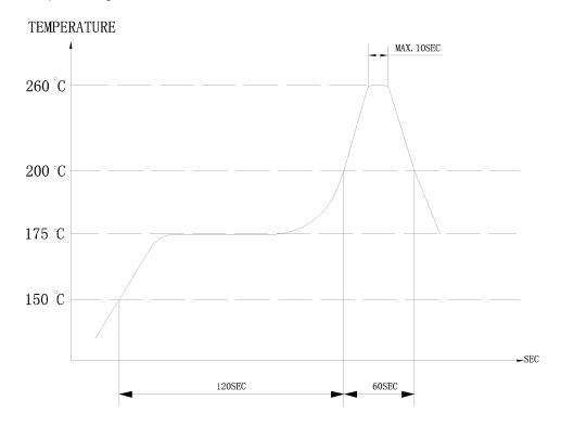
Heat resistant line (Used when heat resistant reliability test is performed) (2)Manual soldering
